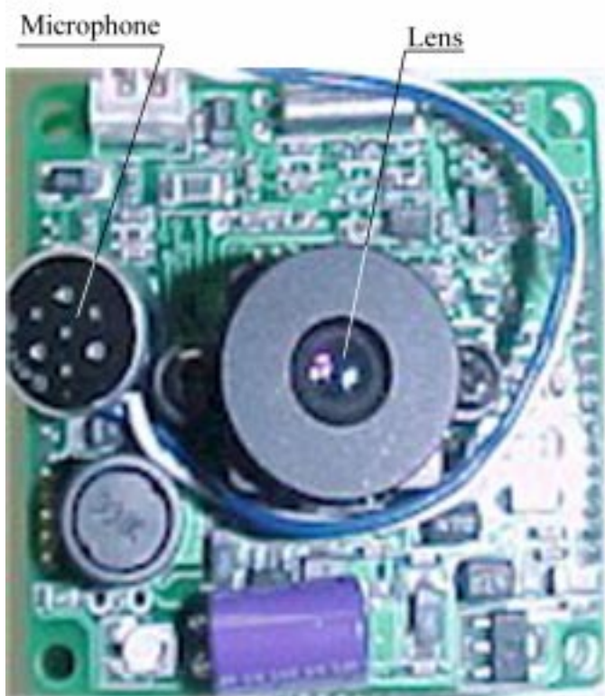
Figure 8. Example of a board camera
